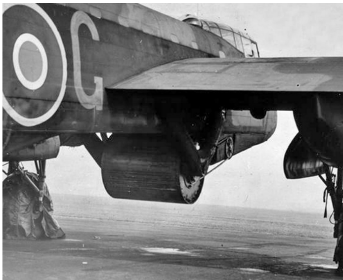
"Upkeep" Bouncing Bomb mounted under Gibson's Lancaster AJ-G 'G for George'. Image-IWM.
