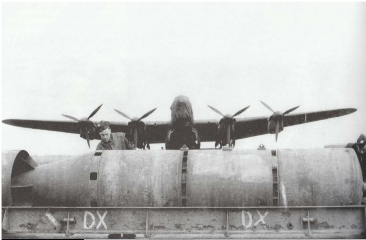
A 12,000 lb HC bomb being made ready for loading in front of JB-144 KC-N at Scampton. Image from Dambusters - The Definitive History of 617 Squadron at War 1943-1945 by Ward, Lee and Wachtel.
